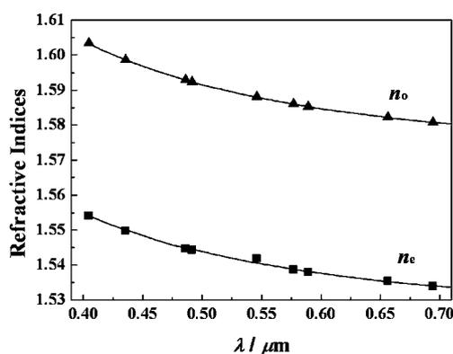
Fig. 6 Refractive index dispersion curves of a KBB crystal. The points are experimental values; curves are the fits given by the Sellmeier equations.
