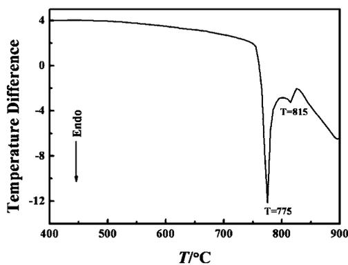
Fig. 1 DTA curve of KBB.
