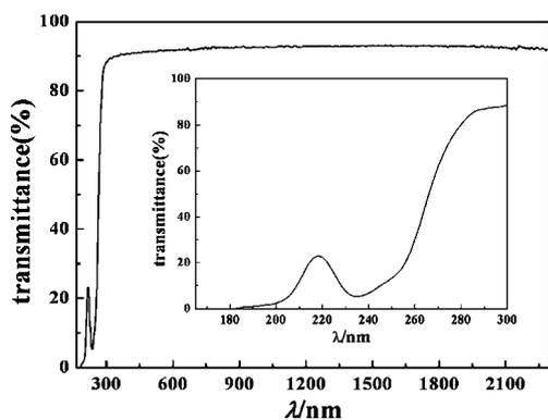
Fig. 5 Transmission spectrum of a KBB crystal. Inset gives the transmittance versus  $\lambda$  curve between 165 and 300 nm.
