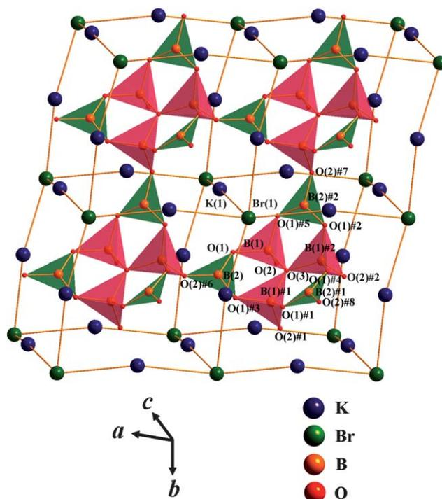
Fig. 3 Drawing of the structure of KBB.  $\text{BO}_4$  tetrahedra and  $\text{BO}_3$  triangles are shaded in red and green, respectively. Symmetry transformations used to generate equivalent atoms: (#1)  $1 - y, x - y, z$ ; (#2)  $1 - x + y, 1 - x, z$ ; (#3)  $x, x - y, z$ ; (#4)  $1 - x + y, y, z$ ; (#5)  $1 - y, 1 - x, z$ ; (#6)  $5/3 - x + y, 4/3 - x, 1/3 + z$ ; (#7)  $2/3 - y, -2/3 + x - y, 1/3 + z$ ; (#8)  $-1/3 + x, 1/3 + y, 1/3 + z$ .
