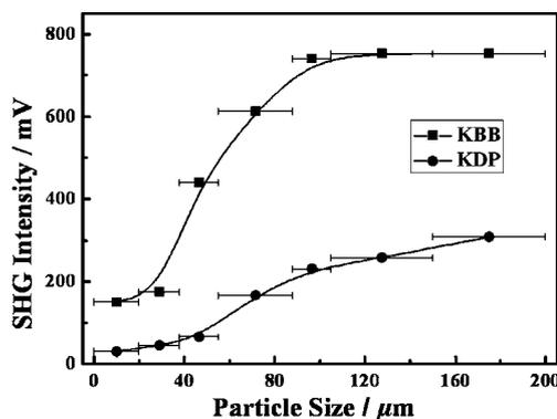
Fig. 4 Phase-matching curves, *i.e.*, particle size vs. SHG intensity, for KBB and KDP. The solid curve drawn is to guide the eye and is not a fit to the data.
