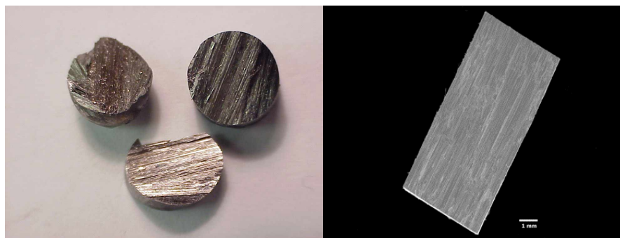
Figure 1. The crystal growth of \text{CsBi}_4\text{Te}_6 perpendicular to the translation axis in a Bridgman furnace is shown in the sliced ingot grown in a cylindrical container (approx 1 cm in diameter) (left) and a sample for TE property measurements was grown by a slow cooling and cut to be a rectangular shape with an approximate dimension of 7 \times 5 \times 5 \text{ mm}^3 (right).
