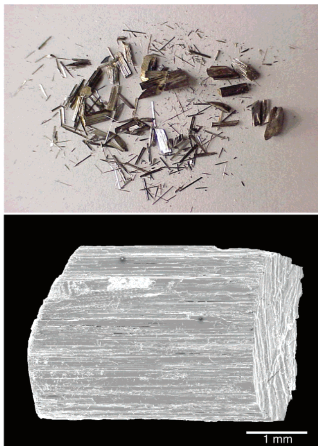
Figure 2. The crystals (top) and oriented ingot (bottom) of \text{CsBi}_4\text{Te}_6 . The direction of crystal growth is the b -axis in the structure.
