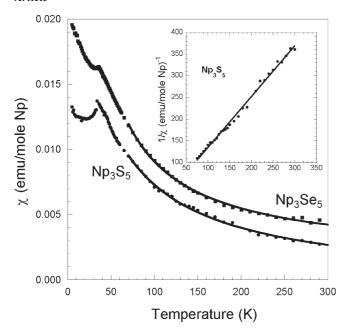
**Figure 3.**  $\chi$  versus T for Np<sub>3</sub>S<sub>5</sub> and Np<sub>3</sub>Se<sub>5</sub> under an applied field of 0.2 T. The solid line through the data above 70 K represents the best fit to the modified Curie-Weiss law. The inset shows  $1/\chi$  versus T for Np<sub>3</sub>S<sub>5</sub>.
