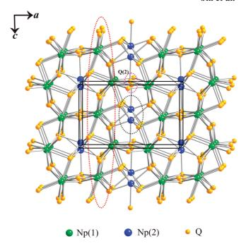
Figure 1. Structure of Np<sub>3</sub>S<sub>5</sub> and Np<sub>3</sub>Se<sub>5</sub>.
