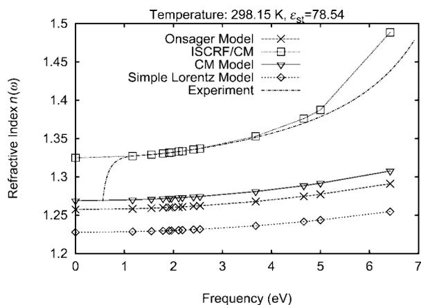
**FIGURE 4.** Dispersion of the refractive index for the best performing ISCRF (Clausius-Mossotti/difference shell) procedure compared with corresponding results obtained from Eq. (7), (8), and (10) using gas-phase polarizabilities. All of these have been evaluated in the difference shell approach with the ANO[432/32] basis set. For the Onsager model ( $\times$ ),  $R_{\text{cav}} = 7.51525$  au, as determined from the corresponding ISCRF procedure, was used in Eq. (10).
