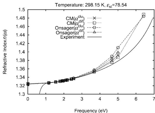
**FIGURE 3.** Dispersion of the refractive index derived from the four different ISCRF procedures as established in this study at 298.15 K. For the ISCRF(Clausius-Mossotti/cluster) and ISCRF(Onsager/difference shell) approaches, the linear response equations could not be converged for the highest frequency, and the corresponding refractive indices are thus omitted.
