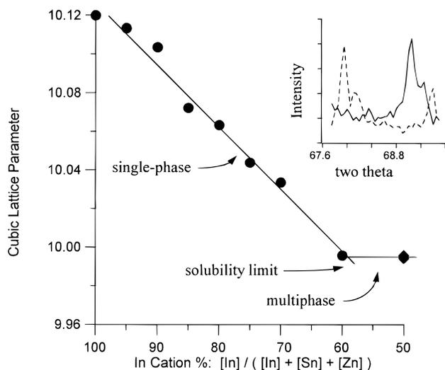
**Figure 1.** Lattice parameter versus cation % In. The sloping region is single phase. The horizontal line is three phase. The inset powder pattern shows the pronounced two theta shift of the 721 peak between In<sub>2</sub>O<sub>3</sub> (dashed line) and In<sub>1.2</sub>Sn<sub>0.4</sub>Zn<sub>0.4</sub>O<sub>3</sub> (solid line).
