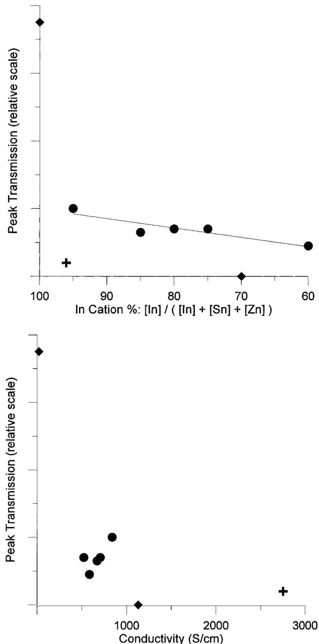
**Figure 5.** Plot of peak (500 nm) transmittance versus cation % In (a, top) and versus conductivity (b, bottom). Samples shown are (◆) cosubstituted copper-quenched including pure In<sub>2</sub>O<sub>3</sub>, (●) air-quenched cosubstituted, (+) 4 cation % Sn ITO.
