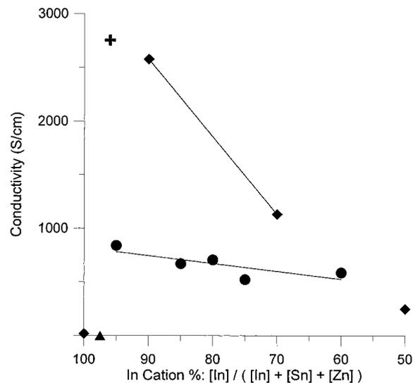
**Figure 2.** Conductivity versus cation % In. Samples shown are (◆) cosubstituted copper-quenched including In<sub>2</sub>O<sub>3</sub>, (●) air-quenched cosubstituted, (+) 4 cation % Sn ITO, (▲) 97.8 cation % In/2.2 cation % Zn oxide.
