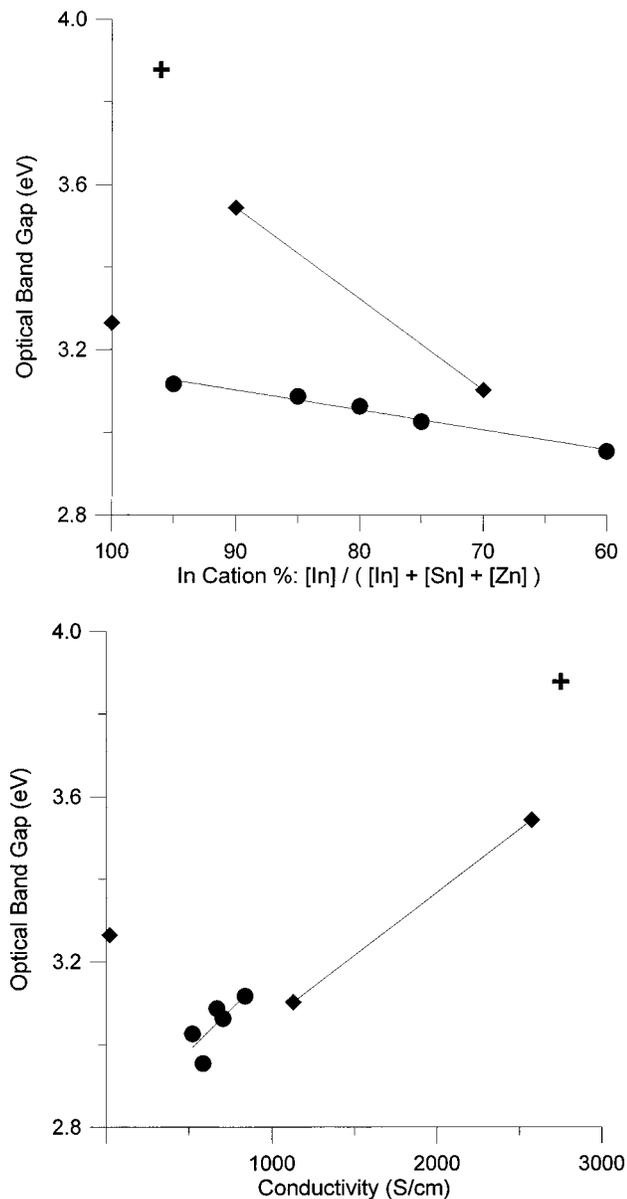
**Figure 4.** Optical bandgap versus cation % In (a, top) and versus conductivity (b, bottom). Samples shown are (◆) cosubstituted copper-quenched including pure In<sub>2</sub>O<sub>3</sub>, (●) air-quenched cosubstituted, (+) 4 cation % Sn ITO.
