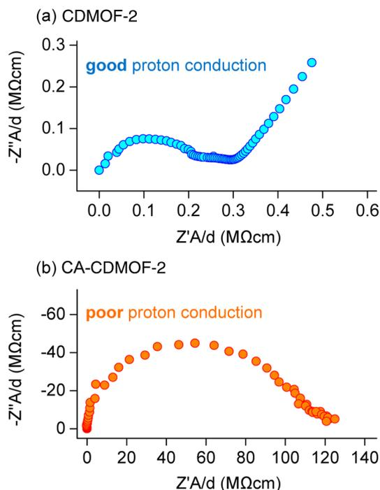
**Figure 2.** Impedance spectra of (a) a pristine CDMOF-2 and (b) CO<sub>2</sub>-infused CDMOF-2 samples following exposure to methanol vapor at room temperature.
