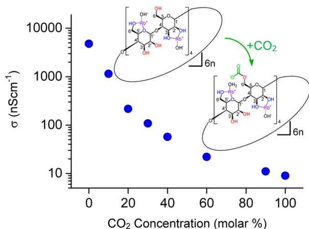
**Figure 4.** Exponential scale plot of average conductivity values in CDMOF-2 samples after their exposure for 5 min to CO<sub>2</sub> gas, which was diluted with N<sub>2</sub> in various concentrations.
