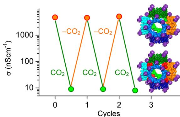
**Figure 3.** Cyclic change of conductivity of a CDMOF-2 sample following sequential CO<sub>2</sub>-sorption and desorption.
