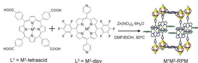
**Scheme 1** Synthesis of **M<sup>1</sup>M<sup>2</sup>-RPM** materials from M<sup>1</sup>-tetraacid, M<sup>2</sup>-dipy and Zn(NO<sub>3</sub>)<sub>2</sub>·6H<sub>2</sub>O. Crystallography derived stick representations of the unit cells of **RPM** (yellow = Zn, red = O, green = F, blue = N, gray = C). Hydrogen atoms and disordered solvent molecules have been omitted for clarity.
